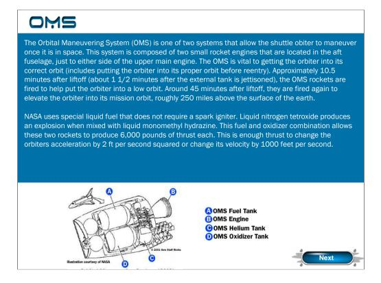
Orbital Maneuvering Subsystem (OMS/RCS) The orbital maneuvering subsystem engine (OMS-E) provides propulsion capability for the orbiter during orbital insertion and deorbit maneuvers. The OMS-E is a 6,000 lbf hypergolic, pressure-fed, fixed thrust engine. There are two OMS engines per orbiter vehicle.
