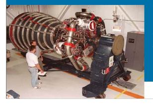
The main oxidizer valve is opened during a propellant dump to allow residual liquid oxygen to be dumped overboard through the engine, and the fuel bleed valve is opened to allow residual liquid hydrogen to be dumped through the liquid hydrogen fill and drain valves overboard. After the dump is completed, the valves close and remain closed for the remainder of the mission
