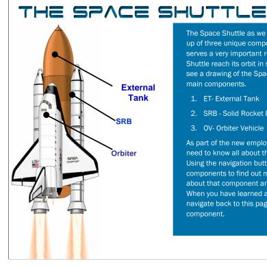
The Space Shuttle as we know it today is made up of three unique components. Each component serves a very important role in helping the Space Shuttle reach its orbit in space. To the left, you see a drawing of the Space Shuttle and its three main components.
