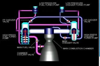
The Low Pressure Fuel Turbopump (LPFT) is an axialflow pump driven by a two-stage turbine powered by gaseous hydrogen. It boosts the pressure of the liquid hydrogen
