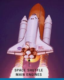
with the Solid Rocket Boosters, provide the thrust to lift the Orbiter off the ground for the initial ascent. The main engines continue to operate for 8.5 minutes after launch, the duration of the Shuttle's powered flight.
